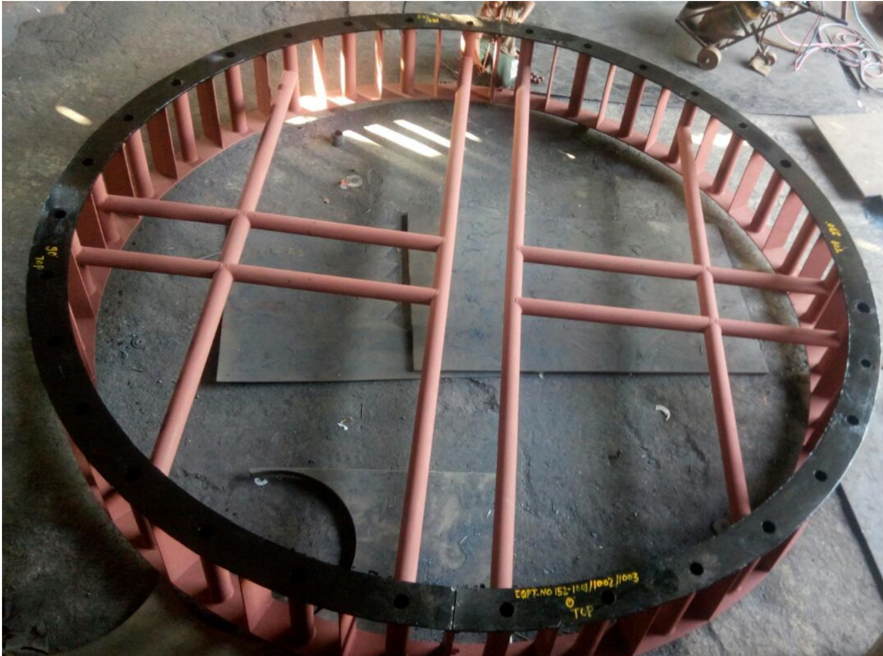
Foundation Ring Template for vertical vessels. Made for Godrej & Boyce Ltd.
